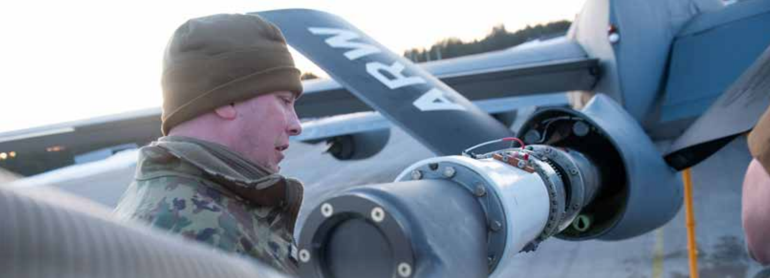
Clockwise from above: Master Sgt. Anthony Lewandowski, a 914th Aircraft Maintenance Squadron airframe and powerplant general flight chief, inspects a drogue installation on a KC-135 Stratotanker. (Senior Master Sgt. Andrew Caya); TSgt. Jared Rogosienski checks instruments on a KC-135 flight deck for an engine run. (Senior Master Sgt. Andrew Caya); Tech. Sgt. Coty Ocke prepares the auxiliary power unit on a KC-135. (Senior Master Sgt. Andrew Caya); Ocke leads a drogue installation on a KC-135. (Senior Master Sgt. Andrew Caya); Tech. Sgt. Michael Randolph and Master Sgt. Moe Shivers, boom operators with the 914th Air Refueling Wing, refuel a Norwegian F-35 Lightning II from a KC-135. (Staff Sgt. Jessica Avallone); Airmen from the 914th Maintenance Group work on their KC-135 Stratotanker during Nordic Response '24. (Senior Master Sgt. Andrew Caya); A Norwegian F-35 Lightning II receives fuel from a 914th Air Refueling Wing KC-135. (Staff Sgt. Jessica Avallone); Randolph checks his instruments before refueling a Norwegian F-35. (Staff Sgt. Jessica Avallone)
