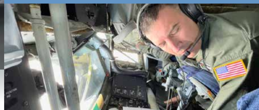
Clockwise from above: Master Sgt. Anthony Lewandowski, a 914th Aircraft Maintenance Squadron airframe and powerplant general flight chief, inspects a drogue installation on a KC-135 Stratotanker. (Senior Master Sgt. Andrew Caya); TSgt. Jared Rogosienski checks instruments on a KC-135 flight deck for an engine run. (Senior Master Sgt. Andrew Caya); Tech. Sgt. Coty Ocke prepares the auxiliary power unit on a KC-135. (Senior Master Sgt. Andrew Caya); Ocke leads a drogue installation on a KC-135. (Senior Master Sgt. Andrew Caya); Tech. Sgt. Michael Randolph and Master Sgt. Moe Shivers, boom operators with the 914th Air Refueling Wing, refuel a Norwegian F-35 Lightning II from a KC-135. (Staff Sgt. Jessica Avallone); Airmen from the 914th Maintenance Group work on their KC-135 Stratotanker during Nordic Response '24. (Senior Master Sgt. Andrew Caya); A Norwegian F-35 Lightning II receives fuel from a 914th Air Refueling Wing KC-135. (Staff Sgt. Jessica Avallone); Randolph checks his instruments before refueling a Norwegian F-35. (Staff Sgt. Jessica Avallone)
